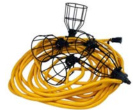
Portable Light Strings Temperature range 60° to -40°C. Sockets every 10 ft w/ coated metal cages Item CEND12012050 (50 ft) • 5 sockets, 12/3 SJT, 600 V Item CEND11912100 (100 ft) • 10 sockets, 12/3 SJTW, 300 V
